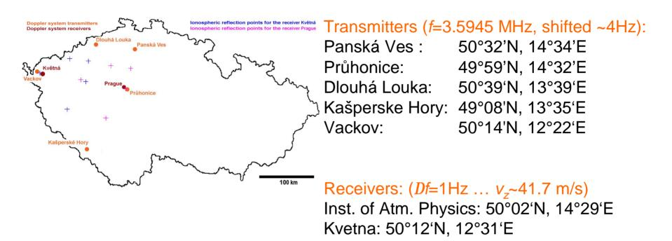
The reflection points are approximately in the mid-points between transmitters and receiver.
